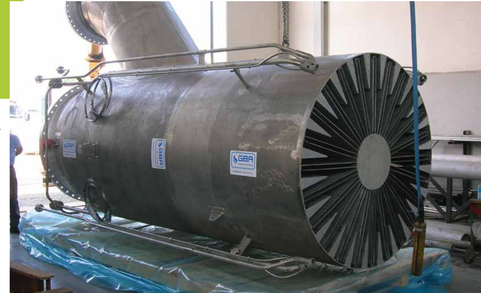
CAF-36-30 Air Assisted Flare Tip Olefins plant
