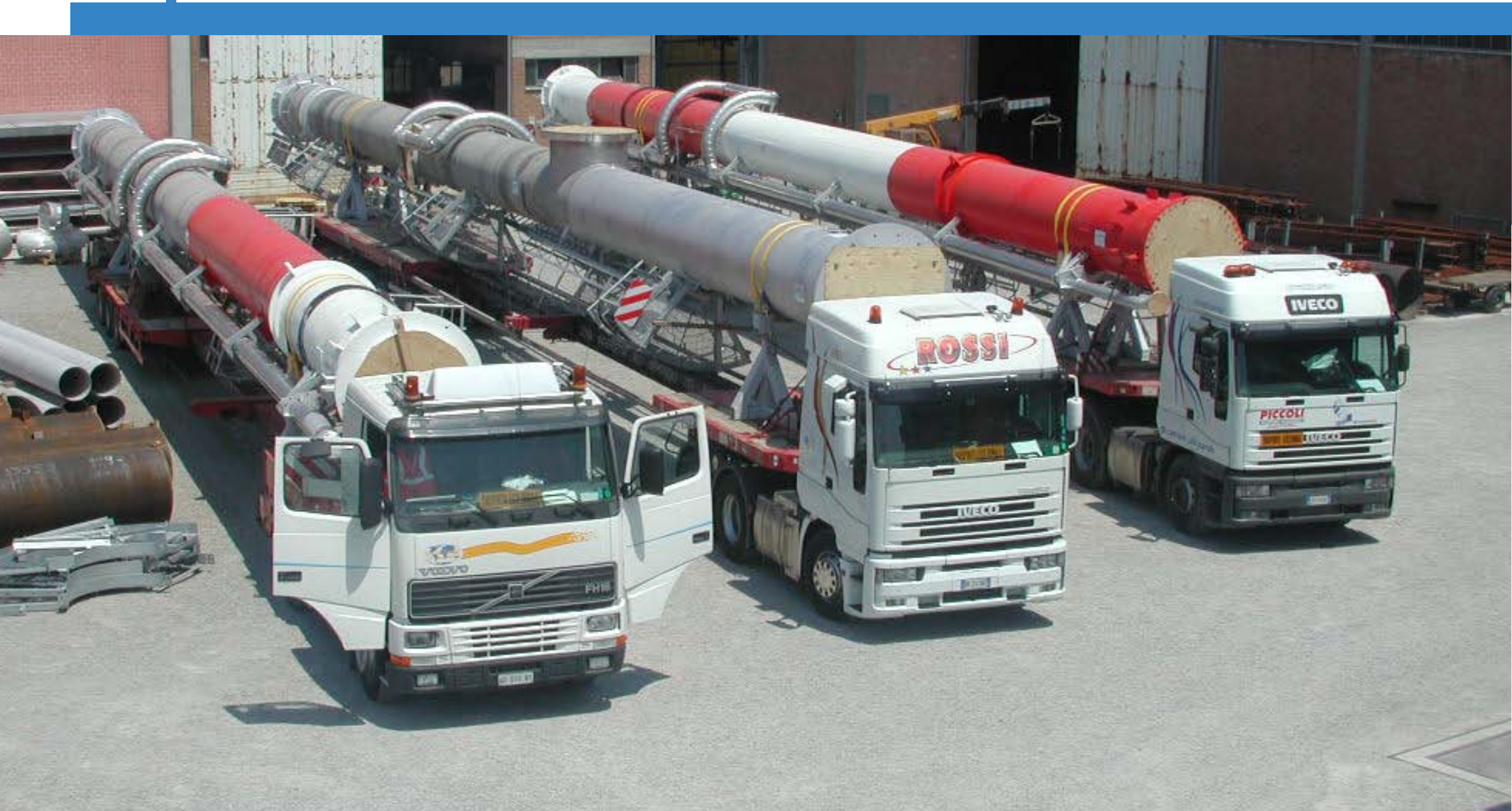
Flare Risers ready for shipping out
