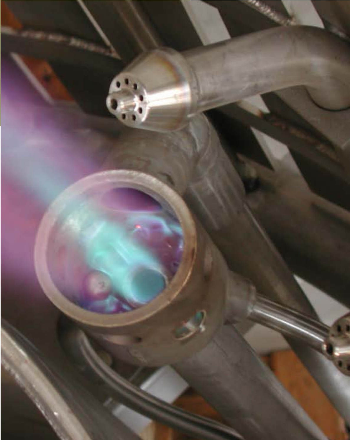
CHT Pilot Nozzle Testing at our works
