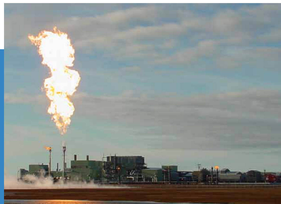
CSF-7-14 Flare Tip Being tested at maximum flow in Alaska
