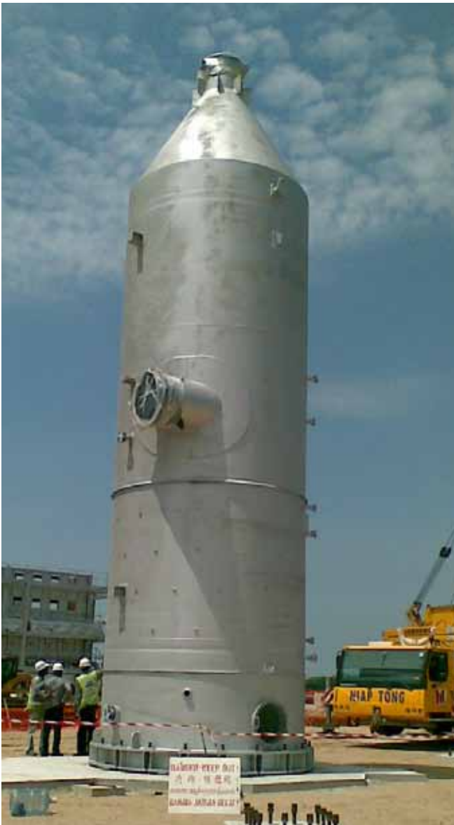
Vertical Knock-out Drum Refinery, Singapore
