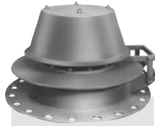
Model 2450 Emergency relief manhole cover with hinged cover with vacuum breaker Sizes: 20" through 24" Vacuum settings: 1/2 OZ./in. 2 to 4 OZ./in. 2 Pressure settings: 2 OZ./in. 2 to 8 OZ./in. 2 Also available pressure only. Page 420
