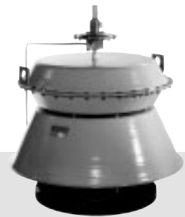
Model 2500 Emergency Relief Valve Sizes: 18", 20" and 24" Pressure settings: 8 OZ./in. 2 to 15 PSIG
