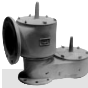
Model 1220 A Pressure/Vacuum Relief Valve Pipe-away feature Modular design Sizes: 2" through 12" Pressure settings: 1/2 OZ./in. 2 to 15 PSIG Vacuum settings: 1/2 OZ./in. 2 to 12 PSIG Page 120
